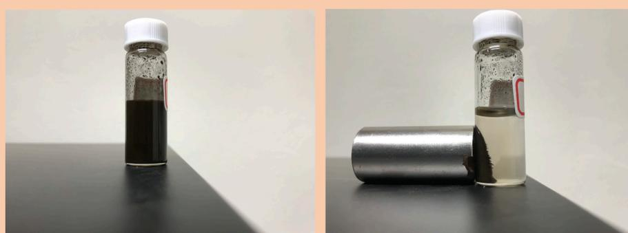
Figure 5. (左)磁性奈米粒子溶液 (右)磁鐵吸附
