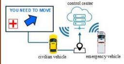
When an emergency vehicle approaches about 300 meters, it transmits information to the server. The AI will retrieve the driver's location, calculate the optimal route, and send To allow the yellow vehicle to yield it to the vehicle's heads-up display. The heads-up display will then instruct the driver on the direction to yield and indicate the lane where the emergency vehicle will pass.
