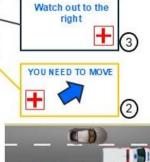
Since the black vehicle does not need to yield, the headsup display will only show the direction the emergency vehicle will pass through.
